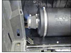
18. Install the provided coupler hose (084055) onto the filter adapter and secure with the provided hose clamp.
