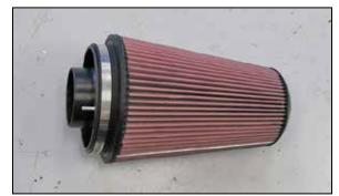
14. Install the adapter assembly into the K&N $^{\rm @}$  air filter and secure with the provided hose clamp.
