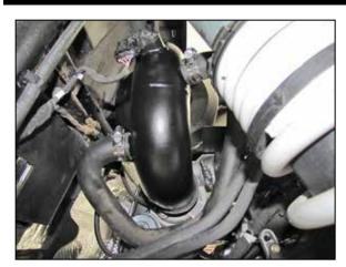
22. Install the K&N® intake tube into the coupling hoses, align for best fit and then secure with the provided hose clamps. Reconnect the inlet temperature sensor electrical connection and connect the BOV hose and crank case breather hoses. Secure the hoses with the provided hose clamps.
